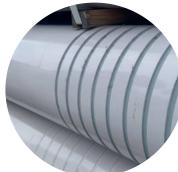
The bottom section of the EcoPile that is driven into the ground has a series of spiral rings cut into it that allows sand to grip the piling better. The extra surface area from the grooves and webs make the EcoPile very resistant to settling as well.
