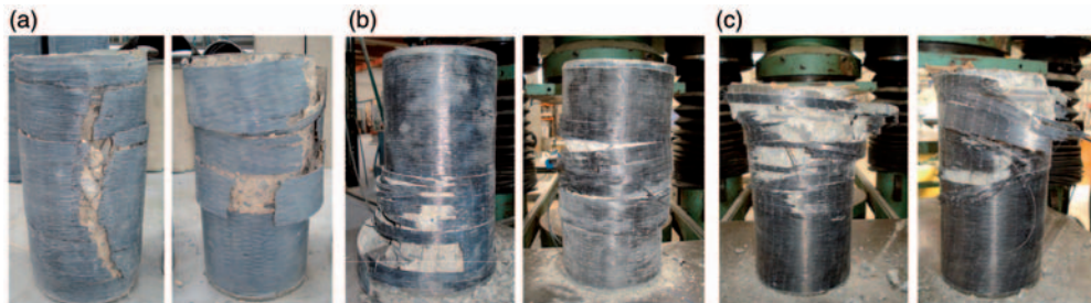
Figure 5. Typical failure modes of CFRP-confined concrete cylinders: (a) f'_{co} = 26 MPa; (b) f'_{co} = 50 MPa; and (c) f'_{co} = 62 MPa.
