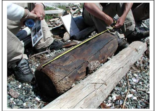
Creosote laden wood is easily identified and removal is clearly achievable. Creosote wood can be systematically identified, measured and recorded using trained work crews or volunteers. Removal can occur in different ways - either hand carried upland, loaded on barges in the water or placing them in slings and carried out by helicopter. The preferred method for disposal is to transport them to the hazardous waste facility.
